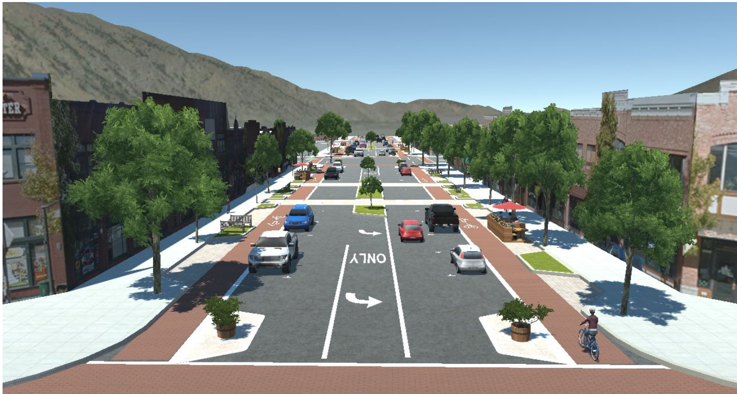
5 Design Alternatives for Main Street, Hailey, ID 5: Rightsizing/Road Diet– 3-Lane w/ Dedicated Bicycle Access
